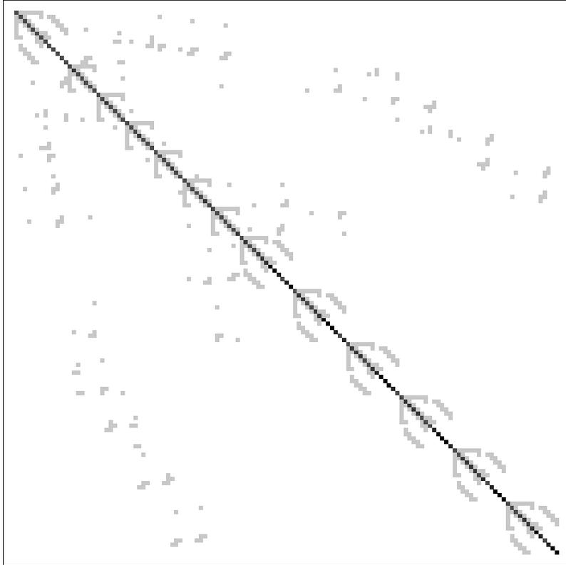
Fig. 4. Structure of the level 2 Laplacian matrix
