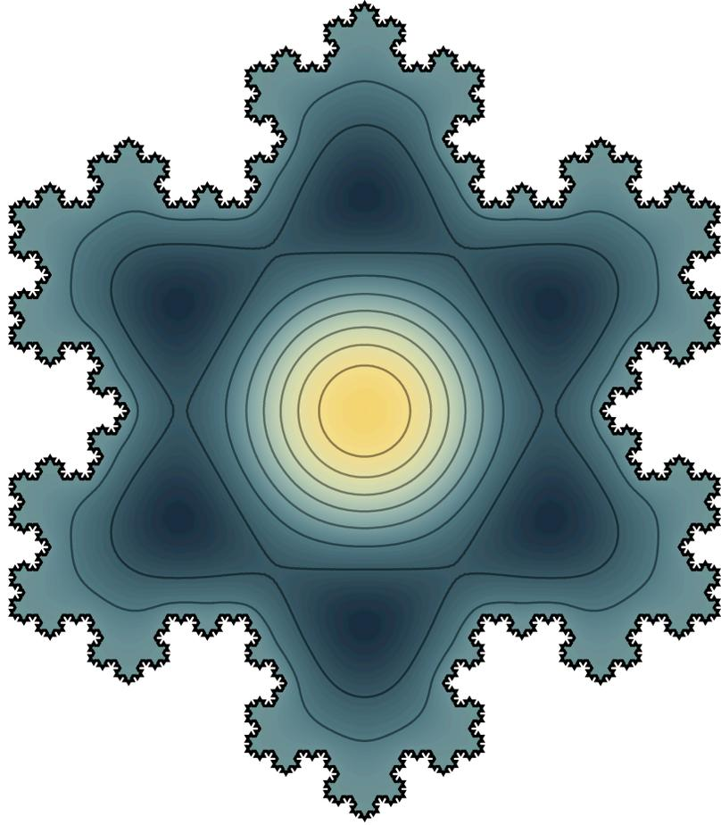
Fig. 7. A contour plot of the sixth mode of vibration
