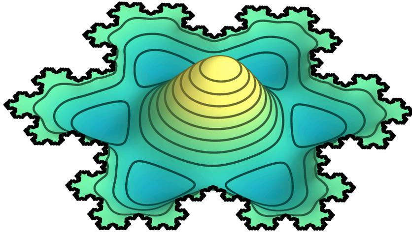
Fig. 9. A 3D plot with contours of the sixth mode of vibration
