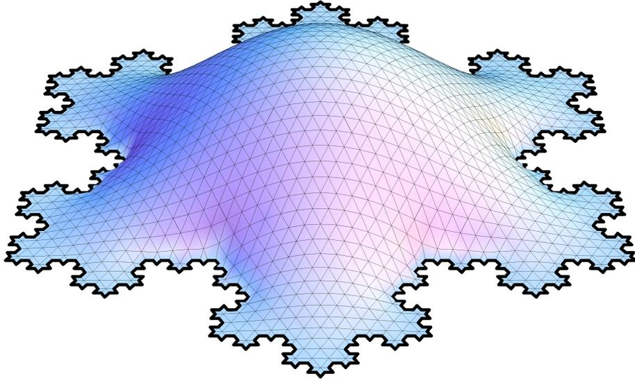
Fig. 5. The lowest frequency mode of vibration
