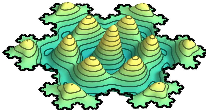
Fig. 10. A 3D plot with contours of the 38<sup>th</sup> mode of vibration
