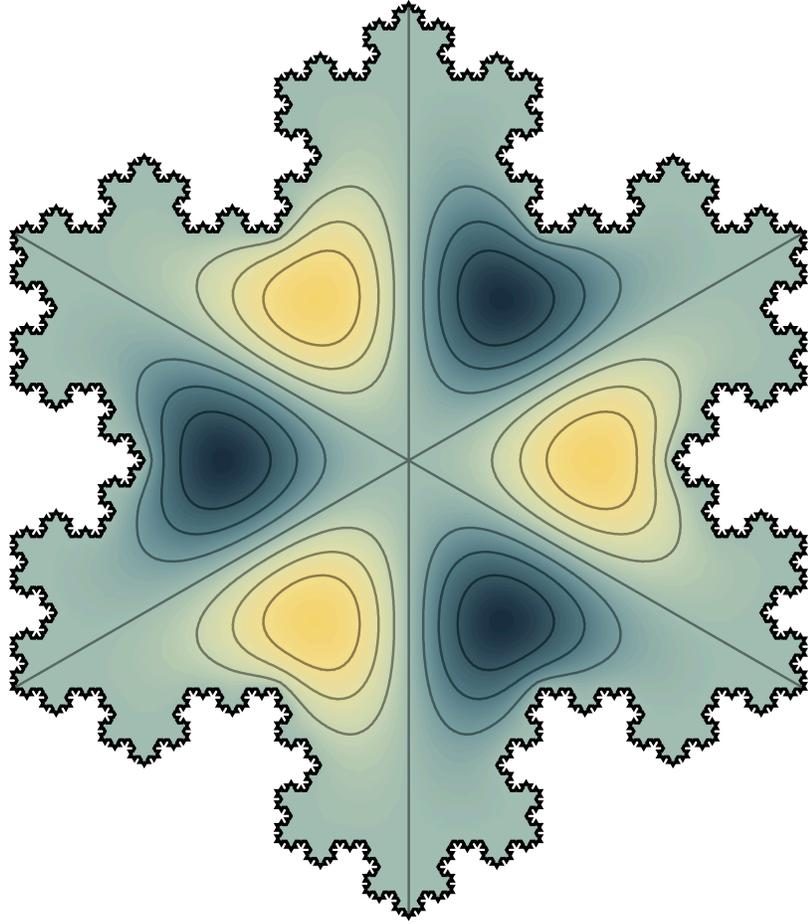
Fig. 8. A contour plot of the tenth mode of vibration
