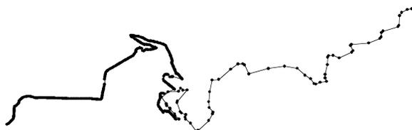
This path exhibits characteristics common to GPS data. Reception is very good in some spots but not so in others. In this example, the better reception occurs on the straighter portions of the path. This is exactly the situation the Douglas-Peucker algorithm is built for. The following picture illustrates the result for several choices of the tolerance.
